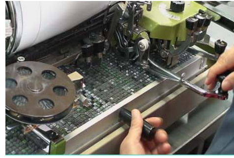
(b) Levers to move the tray and pick up a character.
